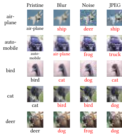
Fig. 1. Illustration of classification results in CIFAR-10. The first column is the pristine sample image of CIFAR-10, whose ground-truth label is on the left and the predicted result is on the bottom of the image. The second, third and fourth columns are the images corrupted by blur, noise and JPEG compression respectively.
